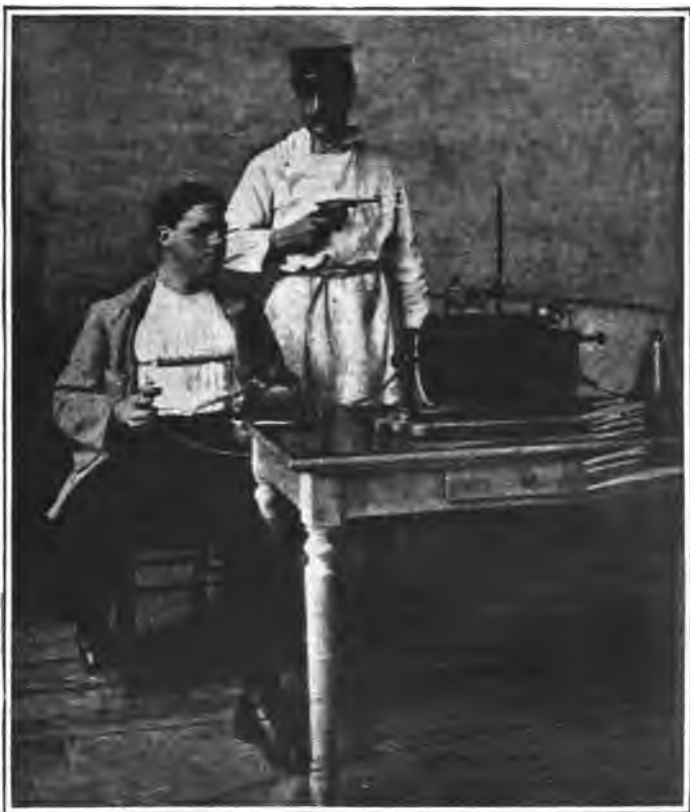
APPARATUS FOR MEASURING TIME REQUIRED FOR REACTIONS AFTER VISUAL, TACTILE OR AUDITORY IMPRESSIONS
